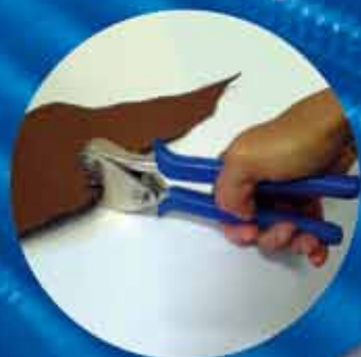
Manual Pliers to mark semi-finished and finished leathers (diam. max 12 mm)
